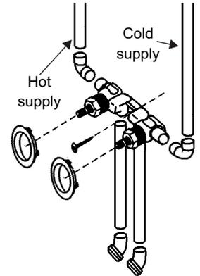
**Step 6.** Connect washing machine hoses to faucet. Turn on water supply and inspect the connections for leaks. Your new Bélanger faucet is now fully installed and ready to use.
