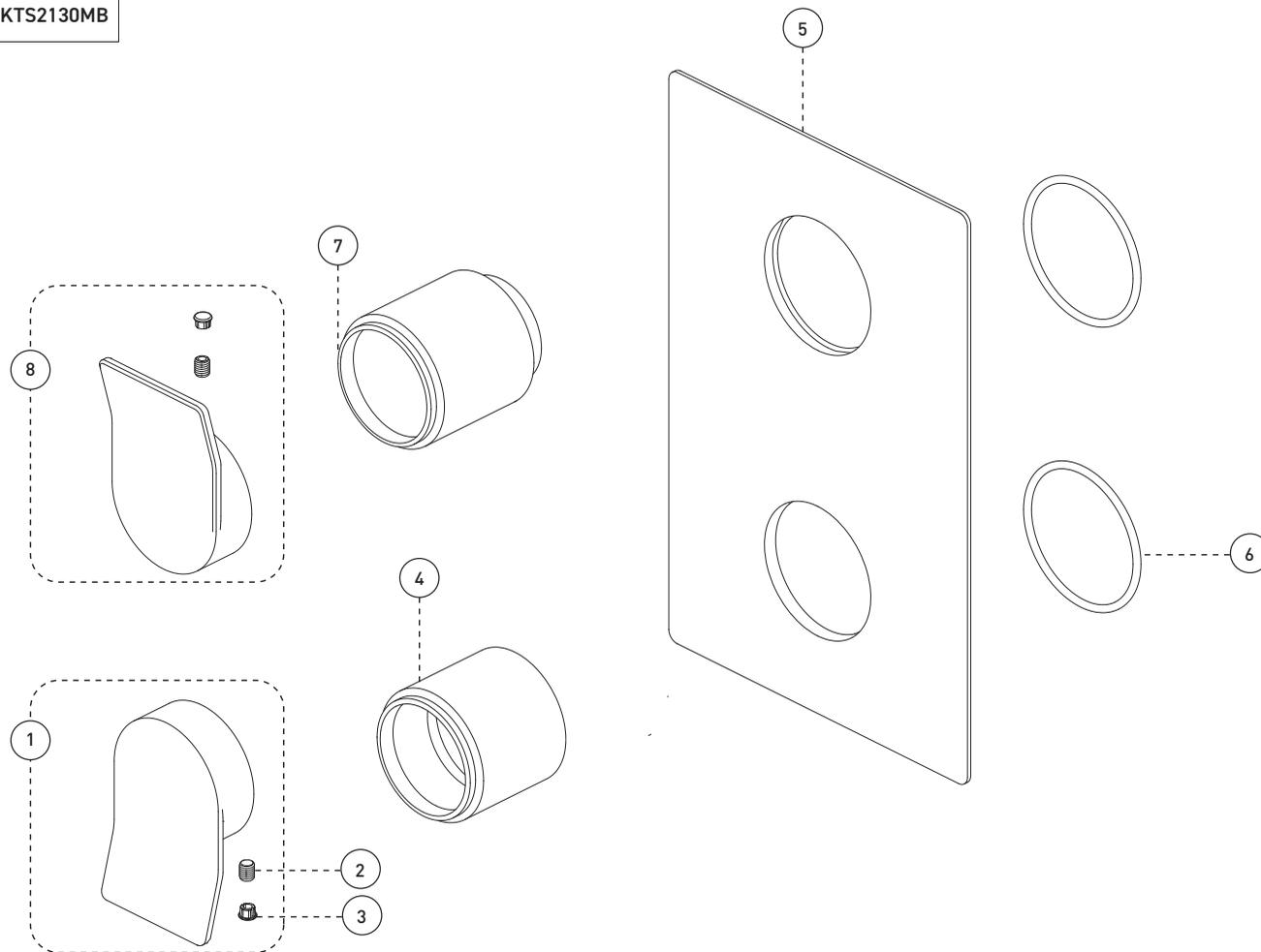
Valve - Trim for Thermostatic 2-way Diverter
