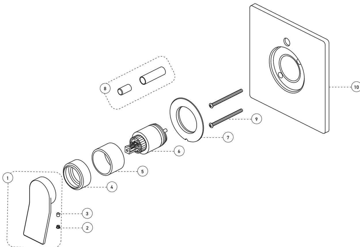
VALVE - TRIM FOR PRESSURE BALANCED DIVERTER VALVE WITH VOLUME CONTROL / VALVE - GARNITURE POUR VALVE À PRESSION ÉQUILIBRÉE, DÉVIATRICE AVEC CONTRÔLE DE VOLUME
