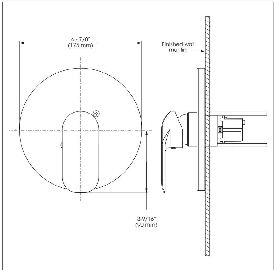
Valve - Trim (T/P) for Pressure Balanced Thermostatic Valve
