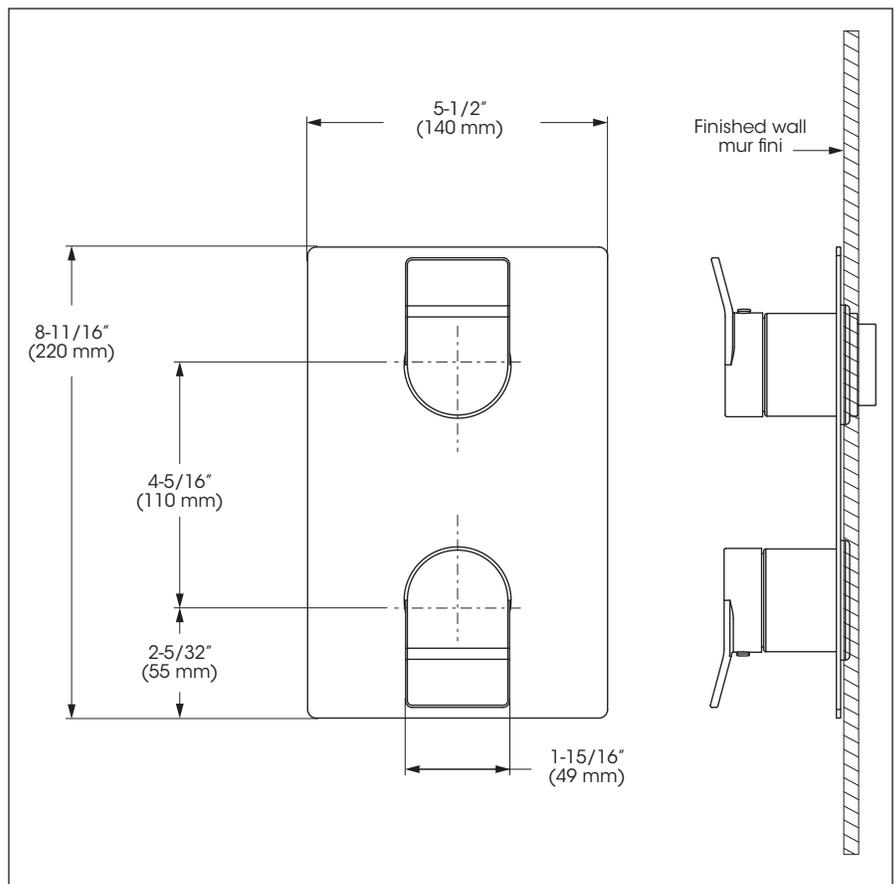
Valve - Trim for Thermostatic 2-way Diverter Valve
