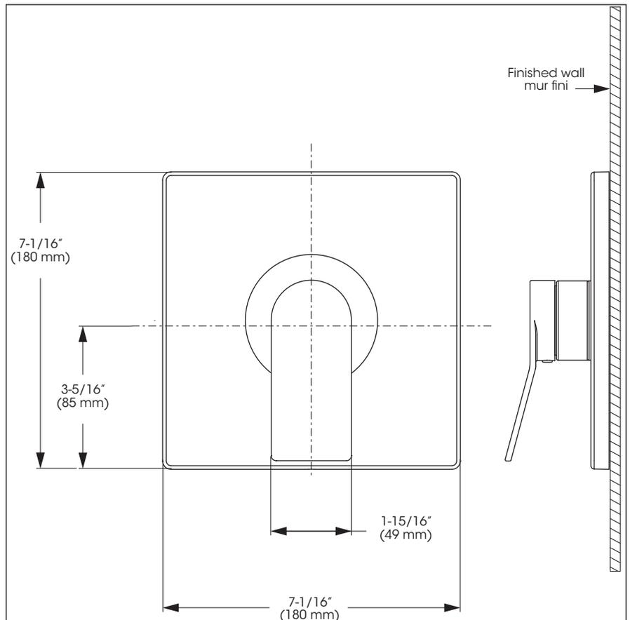
Valve - Trim for Pressure Balanced Valve with Volume Control
